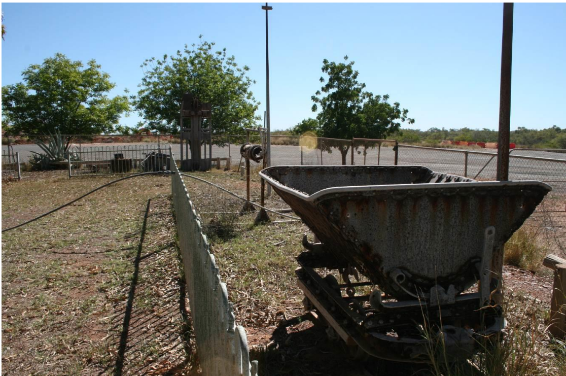
Example of rail wagon used for transporting the ore from the mine to the jetty at Balla Balla, 2012
