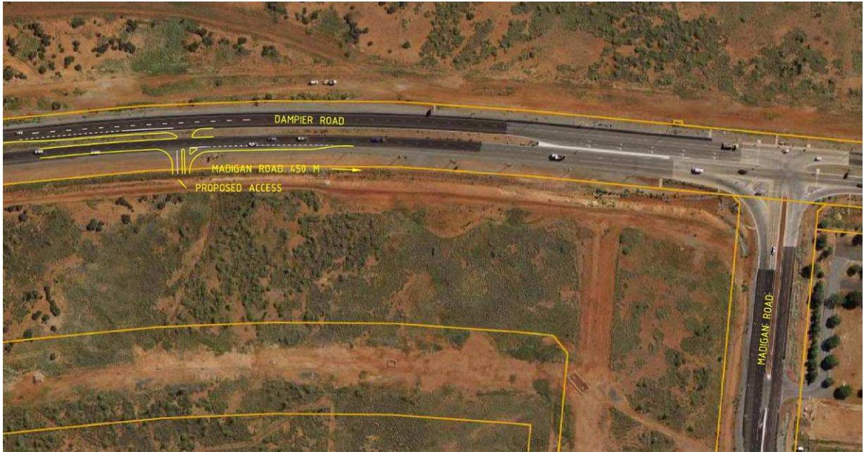
Figure 6. Access Intersection – Concept Geometry
