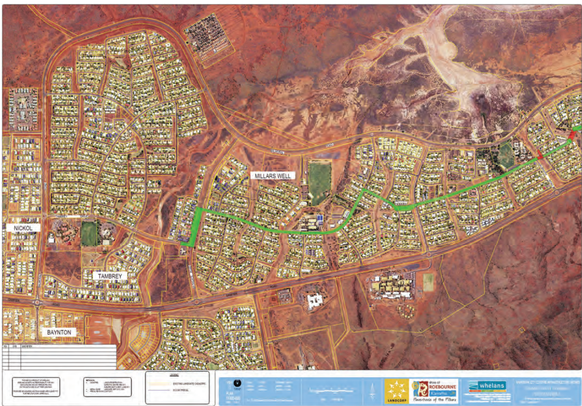
Figure 8 – Preliminary transit plan (west). Green line denotes transit route and red lines new road connections (Source: Whelans, July 2011)
