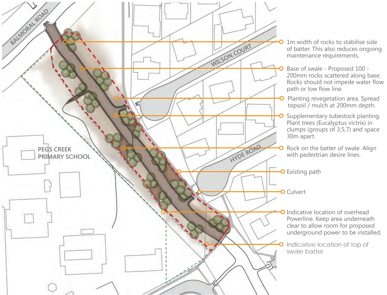
Figure 6.2 Pegs Creek Primary School Swale Plan
